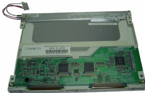
Figure 5-26. LCD Display with Backlight Attached
